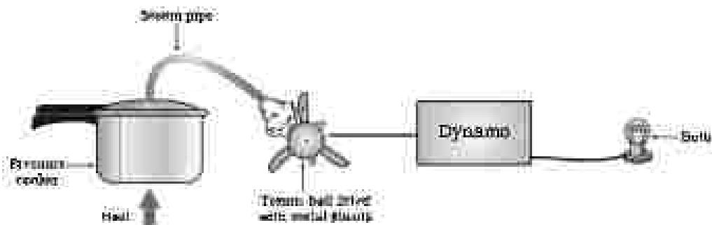
**Figure 14.2 A moving fan dynamo can convert the form of thermal energy into electrical energy!**
