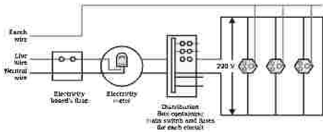
Figure 19.20 A schematic diagram of one of the common domestic circuits.
