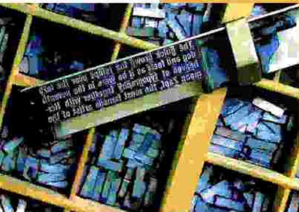
Lead type in compositor trays: (short) type arranged and fixed in a temporary frame
